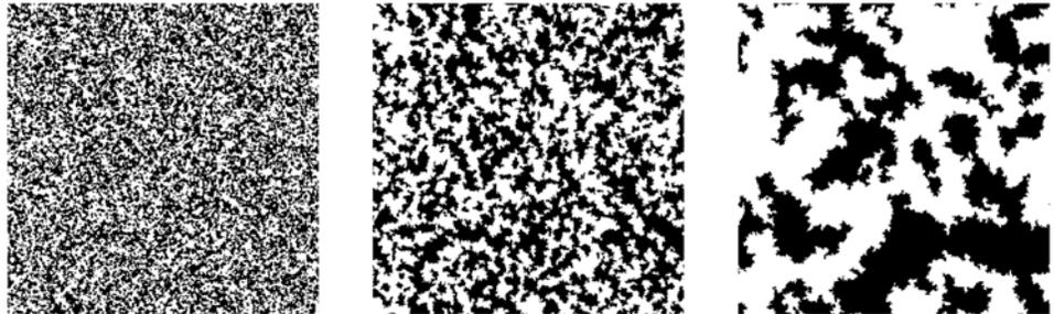
Example coarsening results from patchwork dynamics simulations: spin configurations (as compared with the ground state of the system) after doing patchwork dynamics at various sizes. The system is 512x512 spins. From left to right, the patch sizes used are 2x2, 8x8, 32x32.
