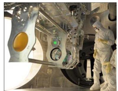
Picture of an Advanced LIGO end test mass suspended by glass fibers (mirror at the far end) and the folded transmission monitor telescope assembly. A glass reaction mass hangs between test mass and telescope assembly which is used as a quiet actuation platform and carries the electrodes for the electrostatic drive. The green light visible on one of the telescope mirrors is used for initial alignment and lock acquisition.
